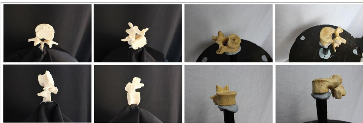
**Figure 3:** Eight different positions of the camera. The first row shows the camera raised by 10 cm from the horizon. The second row is at the horizon. The vertebra was mounted in four different positions. Images presented are examples of those used for reconstruction.
