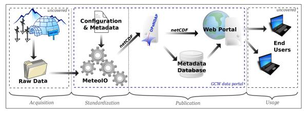
Figure 4: System overview: The raw data are delivered to the data portal where MeteoIO standardizes and OPeNDAP serves the metadata and data to the web portal as NetCDF.
