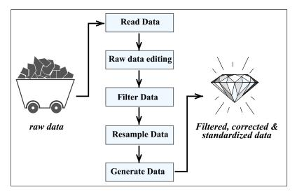
Figure 5: MeteoIO general processing work flow.
