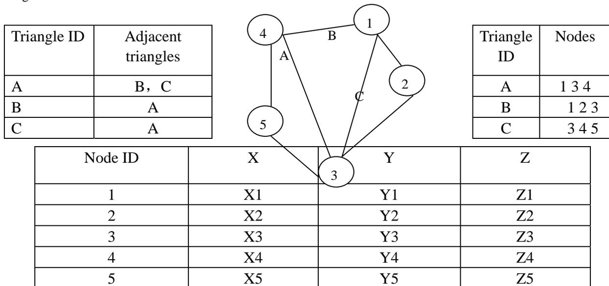
Figure 2. TIN Data Structure
